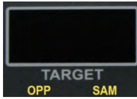
Figure 5.2d OPP and SAME indicator lights
