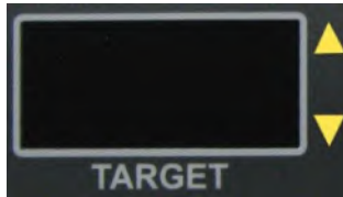
Figure 5.2e TARGET Direction indicator lights
